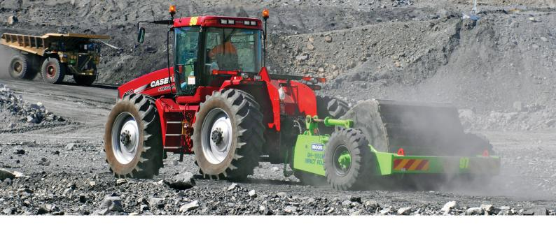
Broons manufactures two Mining Specification versions that have several special features focused on the delivery of cost savings at mine sites. The BH-1300MS has a module 1.3m wide weighing just over 8t.
