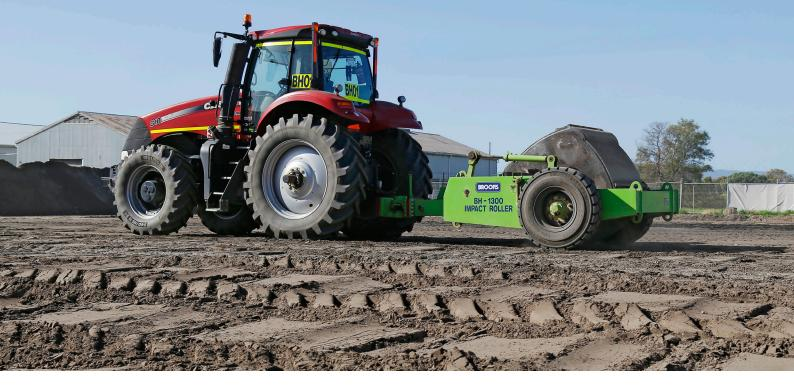
The BH-1300, with its 8 tonne 1.3m wide module, is the original machine developed to deliver rolling dynamic compaction. Significantly upgraded over the years by Broons at their South Australian factory, this work-horse of the fleet continues to deliver cost-effective compaction in a wide range of applications.
