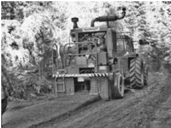
The BH-1220 Rockbuster, a hammer mill crusher that processes windrows of oversized waste rocks and boulders obtained from ditches and road edges.
